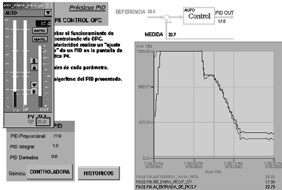
Fig. 11. Main process display of the commented control system.
