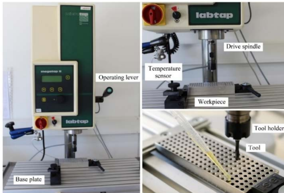
Figure 3. Experimental setup: tribological test using a tapping torque test system with Ti6Al4V workpiece.
