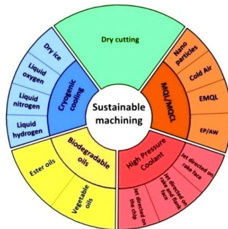
Figure 2. Ring of sustainable machining, reproduced from [50,73], with permission from Elsevier, 2020 and 2019.
