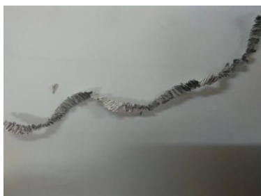
Fig. 8. Chip obtained at 0.05 mm/r and 60 m/min under dry conditions with the tool with a point angle of 118°
