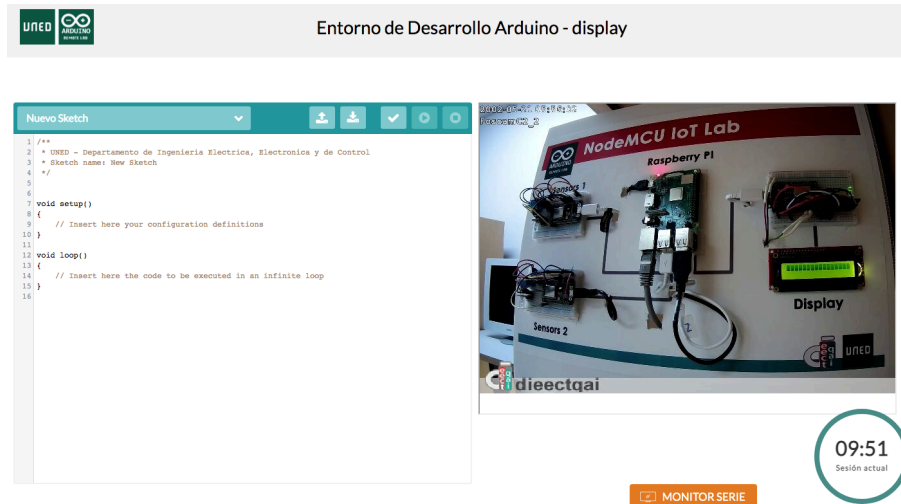
Fig. 2. Screenshot of the web interface of the remote lab, including code editor (left) and webcam video stream (right).
