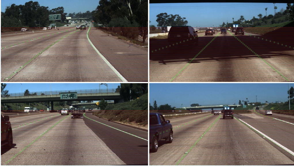
FIGURE 4.1: Example of TuSimple dataset [2]. Even distributed horizontal lines are plotted in red and the intersection with each polyline with a green point.
