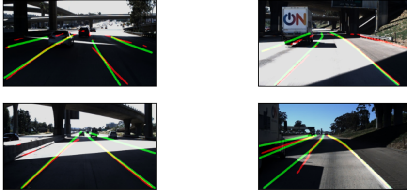
FIGURE 1.1: Lane detection using LaneNet [43] under driving scenarios with shadows, light reflections and lane occlusions from the TuSimple dataset. Green lanes represent the ground truth and red, the one inferred by the CNN.
