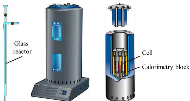
Figure 3.2.4 Glass reactor for adsorption microcalorimetry experiments and Tian Calvet microcalorimeter (Setaram C-80 II) [153].
