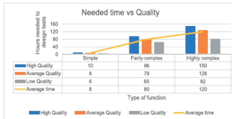
FIGURE 20 Engineering hours spent for test design depending on the type of software module to be validated in black-method
