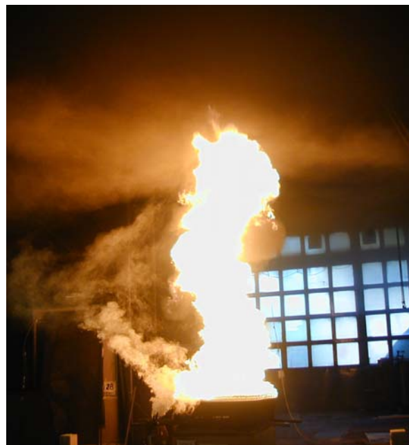
Figure A-24. Photographs of heptane pan fires, ICFMP BE #2, Case 2. Courtesy, Simo Hostikka, VTT Building and Transport, Espoo, Finland.
