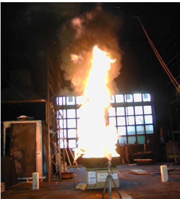
Figure A-24. Photographs of heptane pan fires, ICFMP BE #2, Case 2. Courtesy, Simo Hostikka, VTT Building and Transport, Espoo, Finland.
