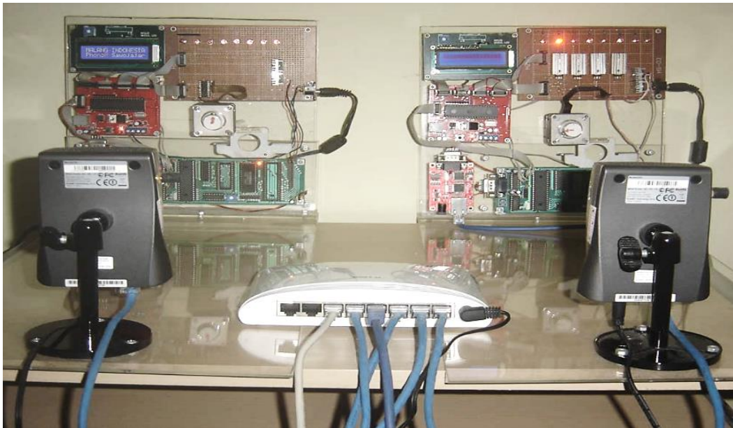
Figure 12. Remote laboratory for programming a microcontroller [37].
